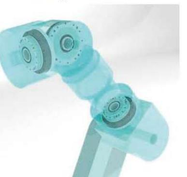
Wafer adsorption handling device
